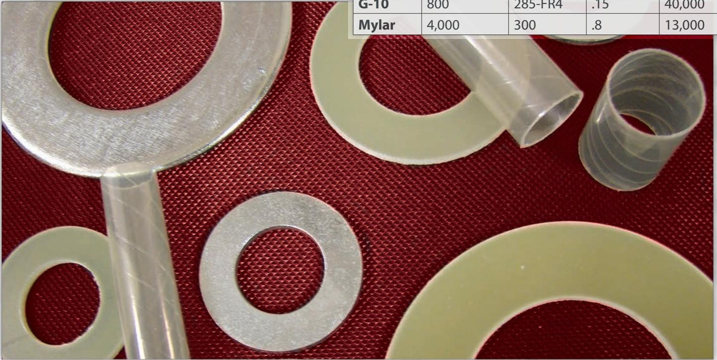
**The G-10 washers** will handle the higher compressive loads as required by the larger diameter bolts and higher pressure rated flanges.
